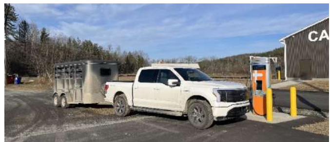
Figure 22: Pull-through charging can accommodate a trailer (Source: Car and Driver)
