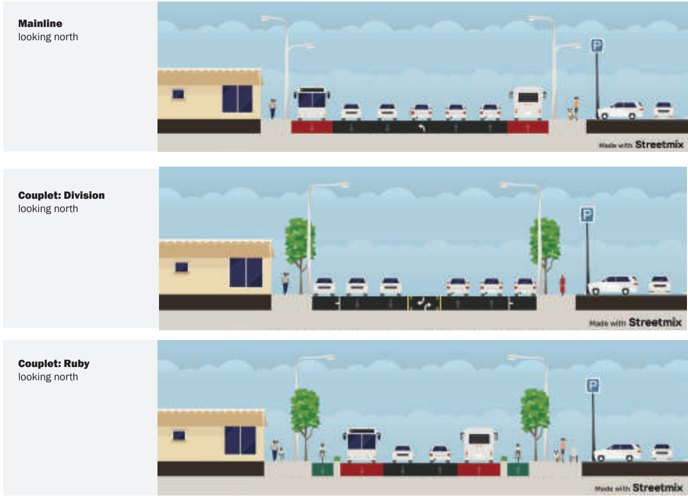
Figure 5-4. Side-Running B Alternative
