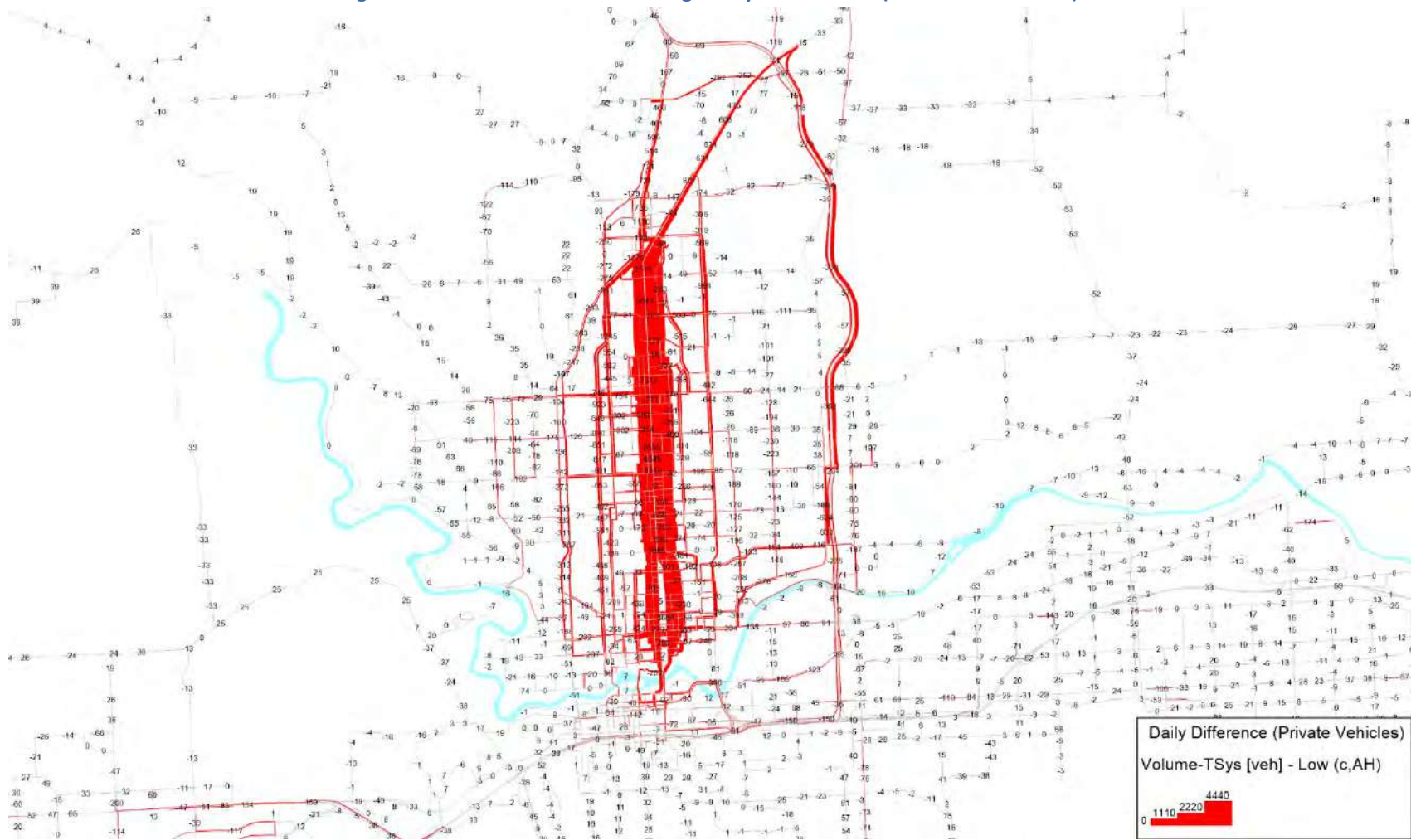
Figure B1: No Build versus Low Average Daily Traffic Flows (No Build Minus Low)
