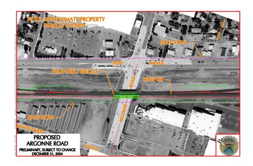
the construction of one additional BNSF mainline track. The additional mainline track is required to move Union Pacific (UPRR) train operations from their mainline corridor into the BNSF corridor. This will allow free movement of freight and commuter vehicles across all railroad mainlines between Spokane, WA and Athol, ID.
