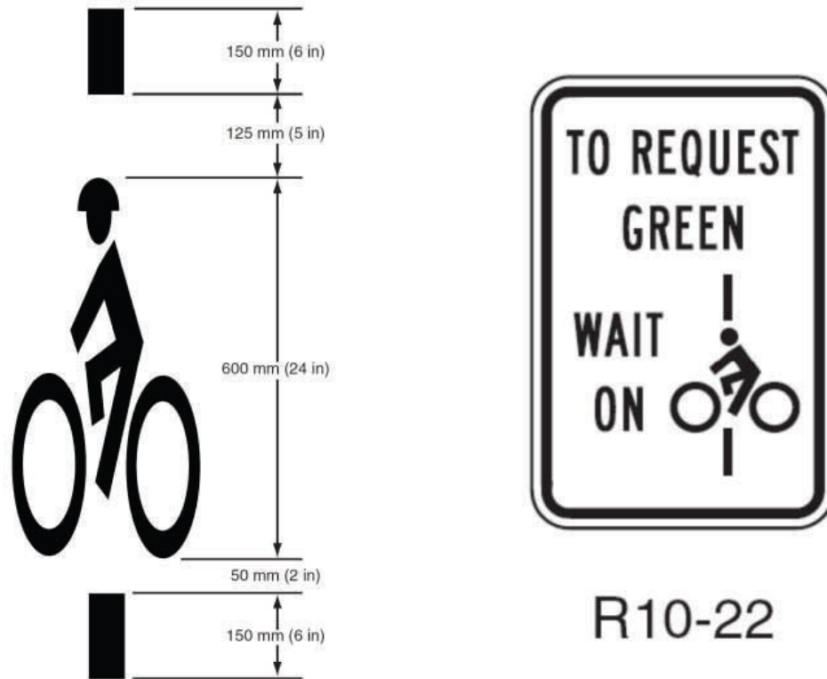
Figure 9C-7. Example of Bicycle Detector Pavement Marking
